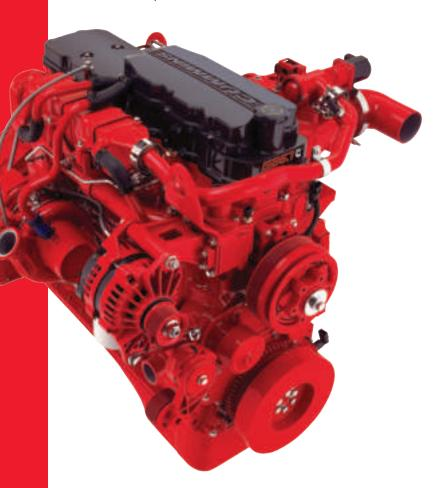
The HPCR fuel system delivers a precise mixture of fuel and air at a constant pressure, regardless of engine rpm. This flexibility in injection timing allows multiple injection events per cycle, which maximizes fuel economy and performance while decreasing noise and exhaust emissions.
